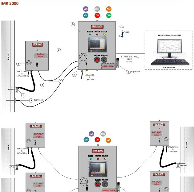
In addition, the IMR 5000 can be equipped to analyze multiple stacks with simultaneous or alternating measurements.
